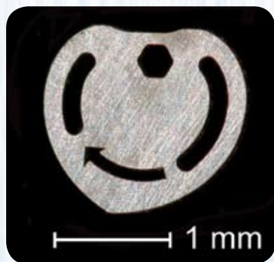
A heart cam manufactured by direct LIGA.
