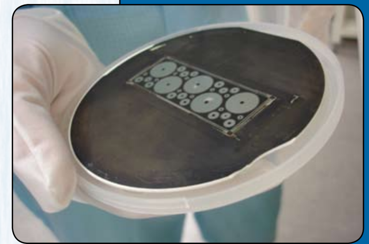
LIGA parts after exposure to X rays in Karlsruhe.
