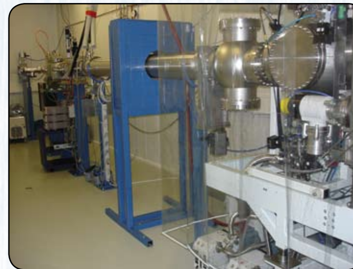
This large machine generates the X-ray light needed to expose the tiny LIGA parts.
